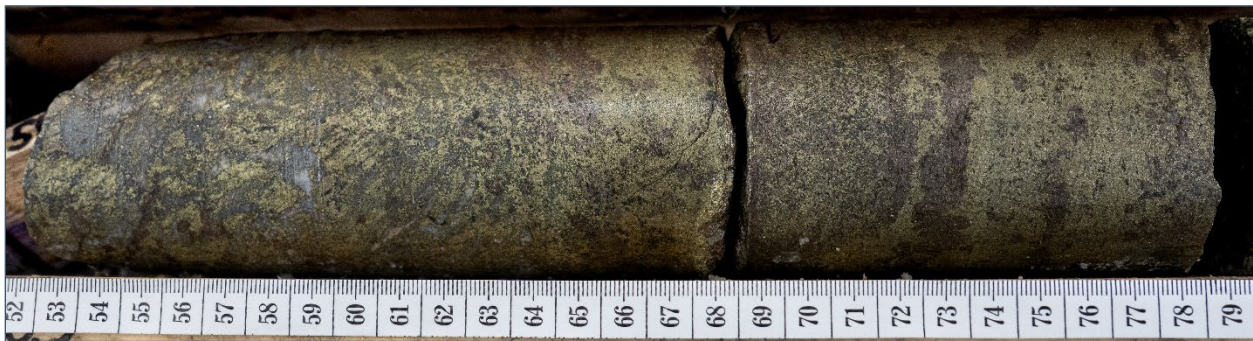
Figure 3. Chalcopyrite-rich interval from CMR26-201 at 350.5 meters i
