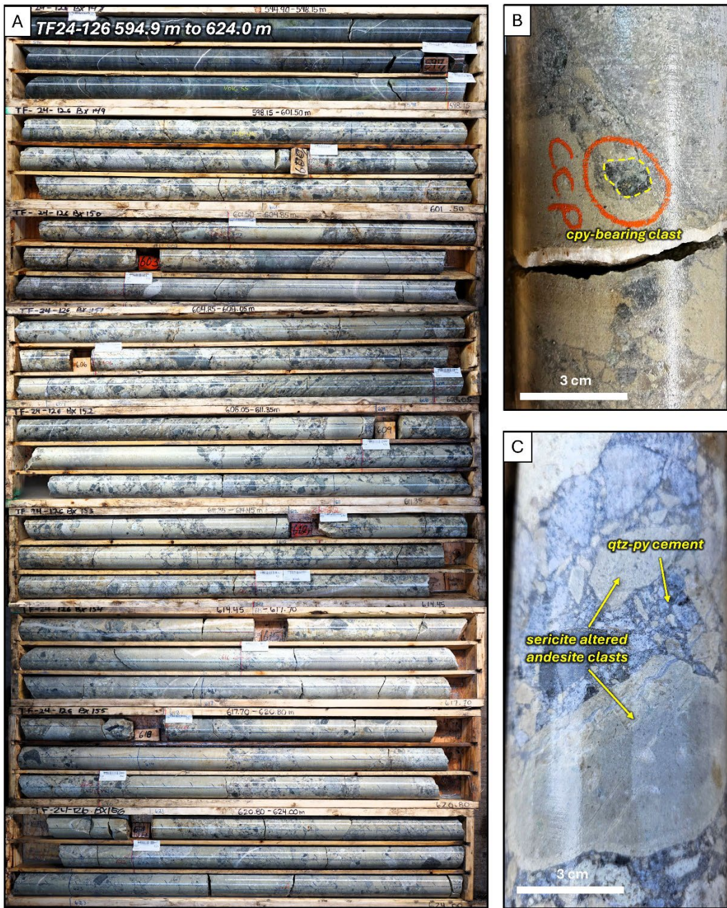
Figure 6. Core photos of the lower breccia zone in TF24-126. A. Box photos showing core from 594.9 to 624.0 meters downhole. Sharp contact with Nicola group volcanics at 598.15 meters. The bleaching of many of the clasts is caused by sericite (white mica) alteration. B. Local chalcopyrite bearing clast in quartz-pyrite cemented breccia. C. Sericite-altered clasts set in a quartz-pyrite hydrothermal cement. Abbreviations: qtz = quartz, py = pyrite, cpy = chalcopyrite.
